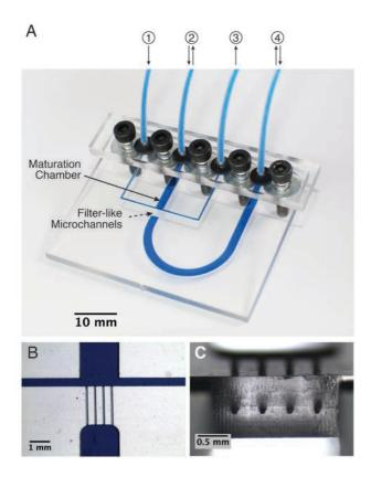
Fig. 4 A) Oocyte-trapping microfluidic device. The dashed arrow indicates the position of the capillary channels that act as a filter for oocytes. For clarity purposes, the channels were filled with blue dye. B) Microscope close-up of the oocyte-trapping region. C) Cross-section view of the oocyte-trapping microchannels embossed using the LTCC master.
