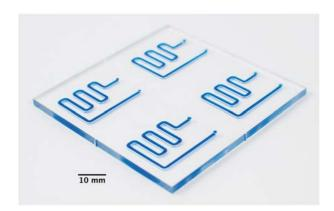
Fig. 3 Microfluidic device for sperm storage. The device features four independent fluidic units to analyze a sample at different times. For clarity purposes, the channels were filled with blue dye.
