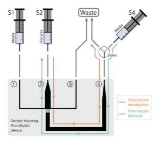
Fig. 2 Schematic representation of the experimental setup for the oocyte maturation experiments *on-chip*. The oocyte-trapping microfluidic device consisted of 4 inlet/outlet ports. Ports 1 and 3 were simply used to fill the device with media and remove any air bubbles trapped next to the filter-like channels. Ports 2 and 4 were used for the oocyte injection/retrieval.
