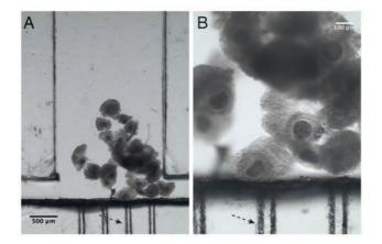
Fig. 5 Microscope pictures of the oocytes trapped in the microfluidic device. The dashed arrow indicates the position of the capillary channels that act as a filter for oocytes. A) General view of the maturation chamber and B) close-up of the oocytes near the capillary channels. The shadowed areas of the capillary channel correspond to its walls, as it has a trapezoidal shape.
